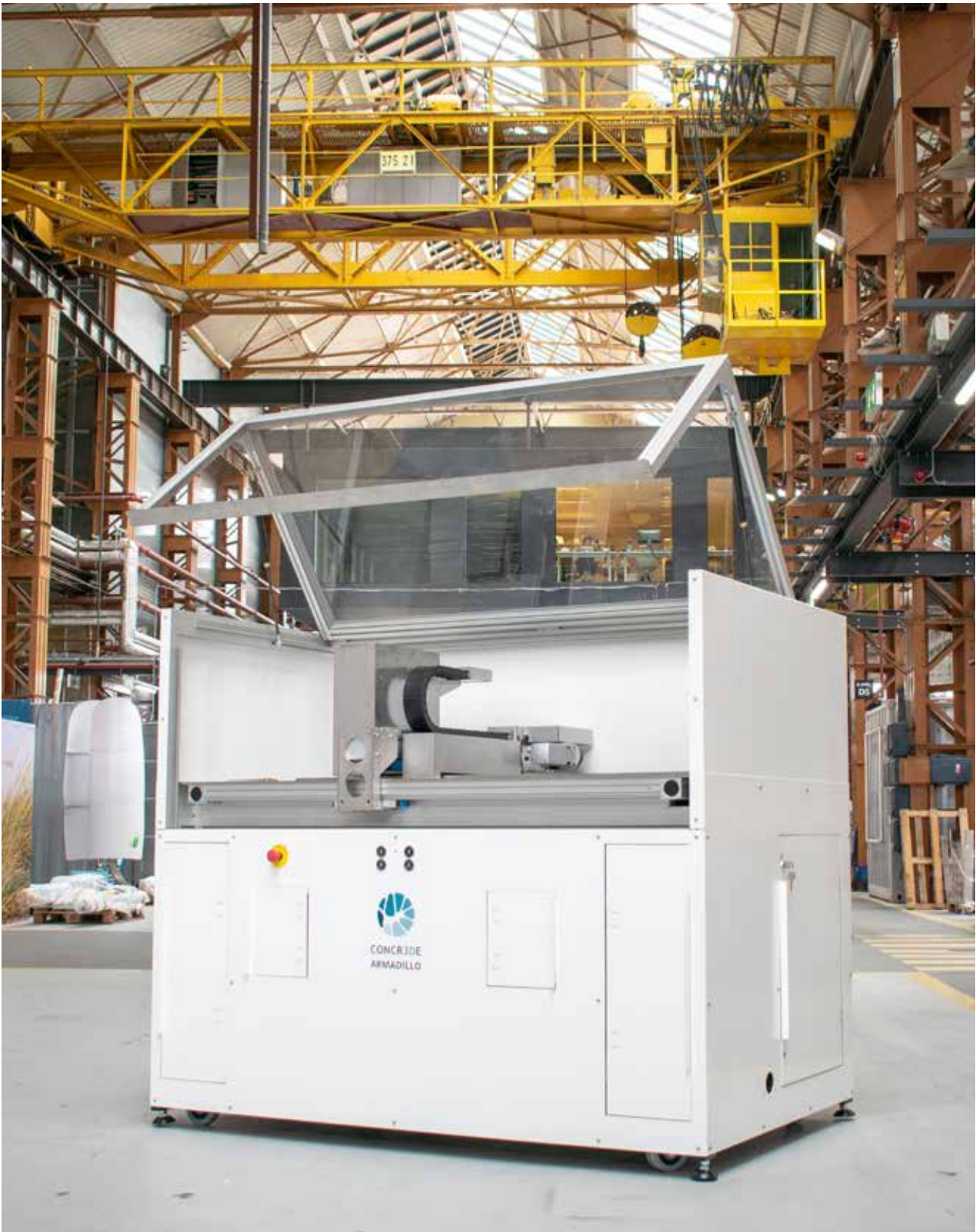
Armadillo White with enlarged printbed, 450x450x250 mm
