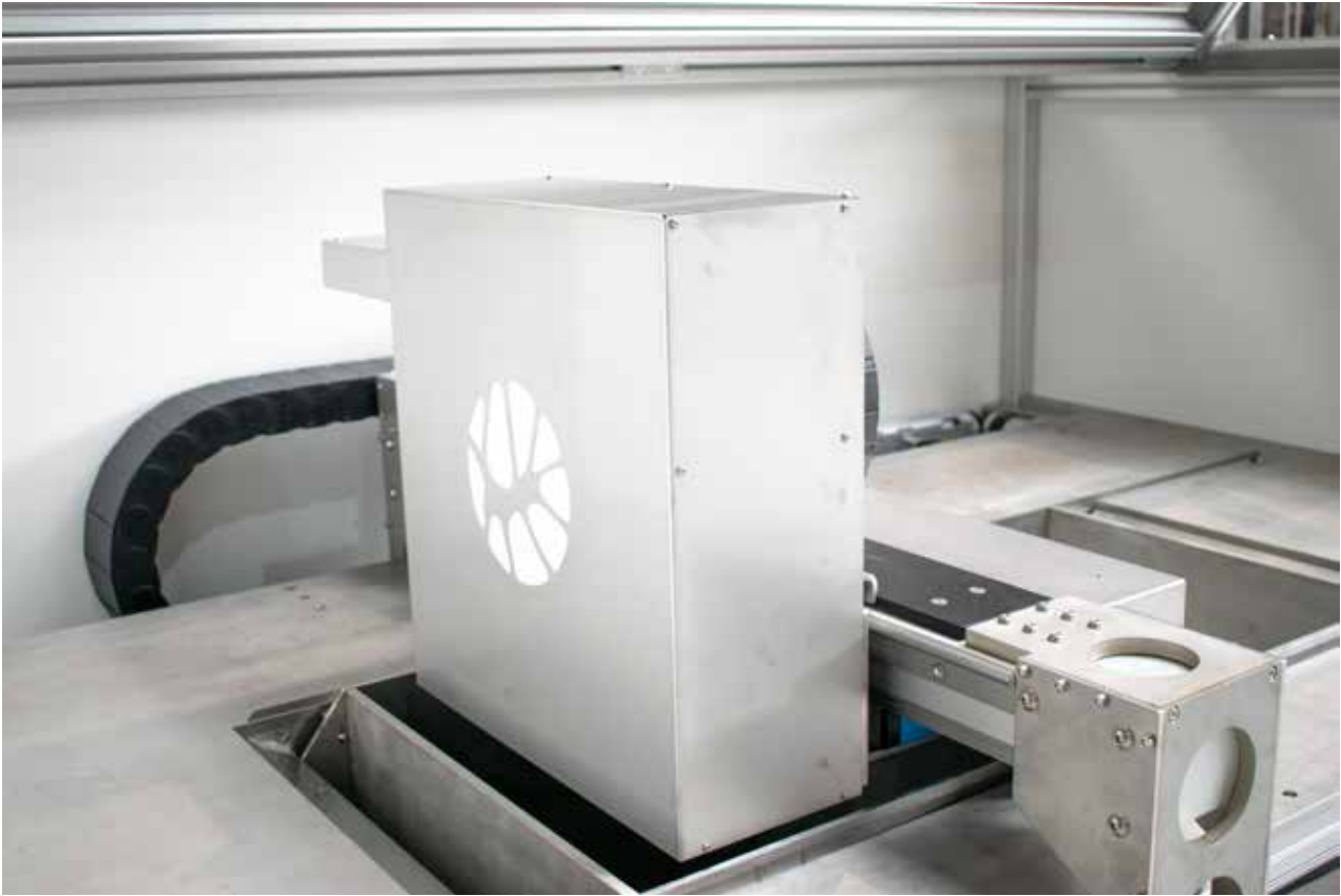
Armadillo White printing system, constructed from stainless steel
